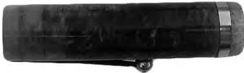
Sheaffer cap with moderate crazing.
